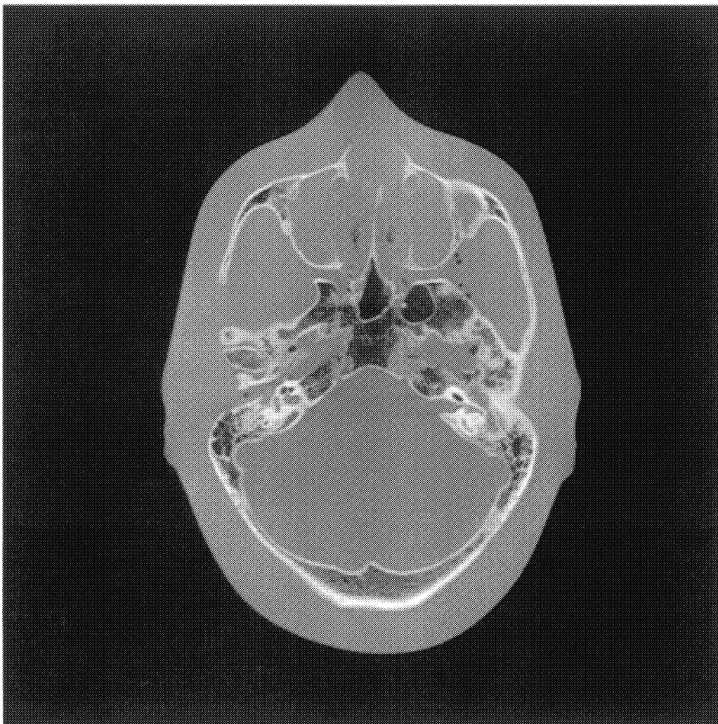
Figure 7. Reconstructed central slice of a head phantom
