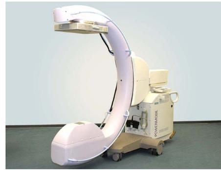
FIG. 1.  $C$  arm prototype with flat panel detector for cone beam CT imaging.
